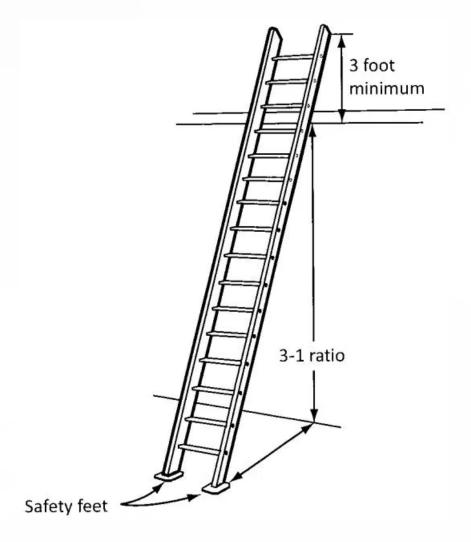
The image shows the proper positioning of a ladder. Ensure the ladder is set 1 ft (30 cm) out for every 3 ft (90 cm) up.
