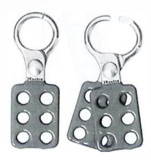
Sometimes more than one person is working on a system or piece of machinery, and since each maintenance worker must use the lockout procedure before starting his or her Chapter, a device called a safety hasp is used to hold the locks. It is attached to the control box of the system or machinery so more than one lock may lock out the power. That way, when one worker is finished, the power remains locked out until the last worker is done.
